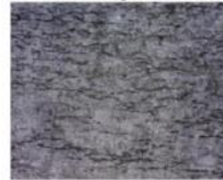
AXLE 057 - EA4T steel - \Delta\sigma = 320 MPa
