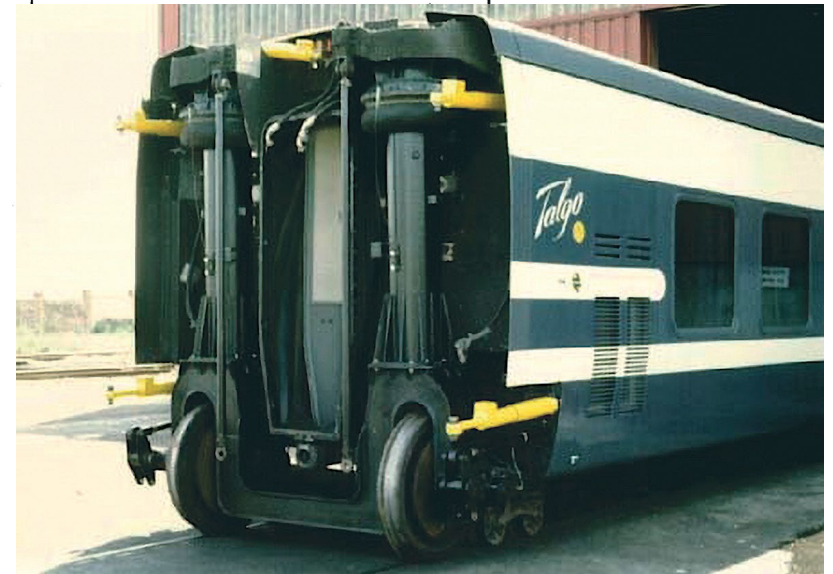
First commercial implementation of natural tilting, Talgo pendular (1980)
