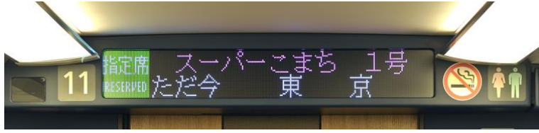
Large annunciator with full-color LEDs
