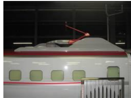
Pantograph and insulation panel
