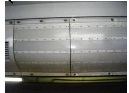
Shroud panels with sound-absorbing panel
